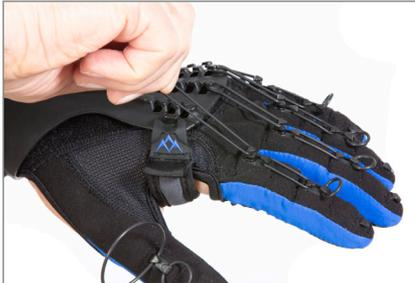
Fig. 31 Reattach MCP Tensioner for all fingers
